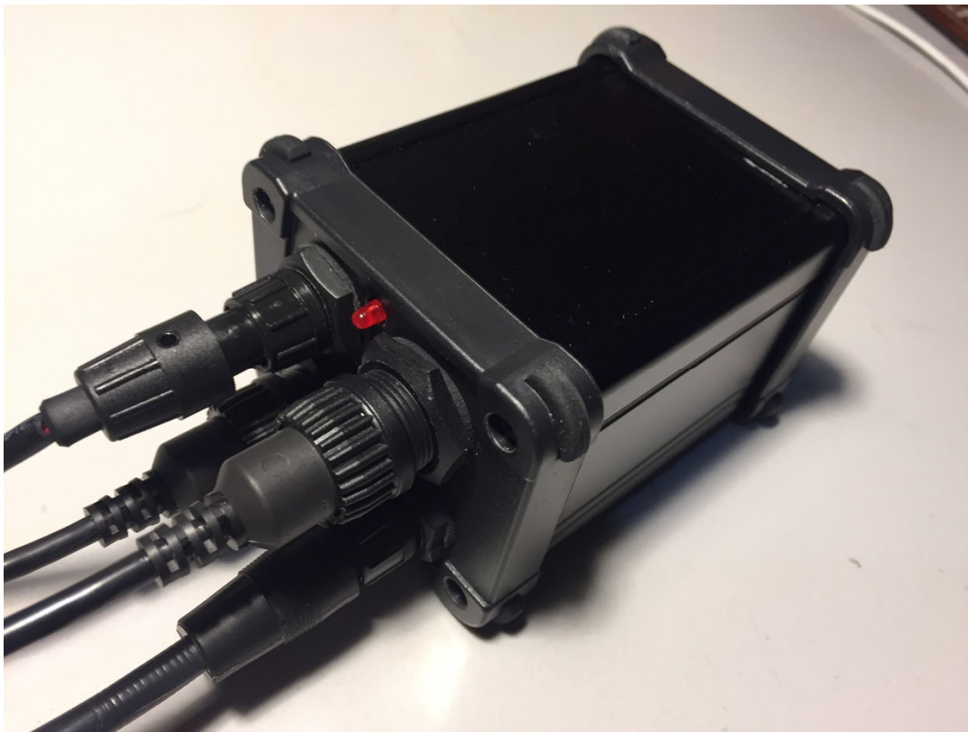
Figure 1: Energy Meter Box
