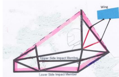
P S E With Wing on Brace
