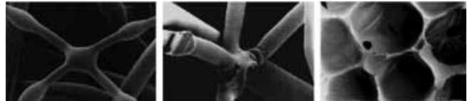
Magnified structure of materials (from left to right) Teijin ELK, PET and PU foam.
