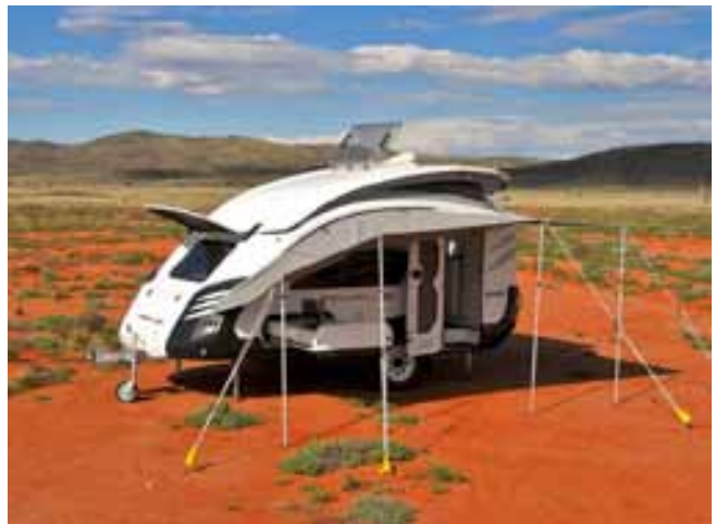
State-of-the-art fibreglass moulding technique delivers a strong, light weight and aerodynamic semi-monocoque unit for the Bolwell Edge Caravan.
