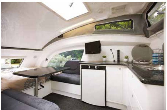
The Bolwell Edge interior fittings are moulded into the inner fibreglass skin of the caravan.
