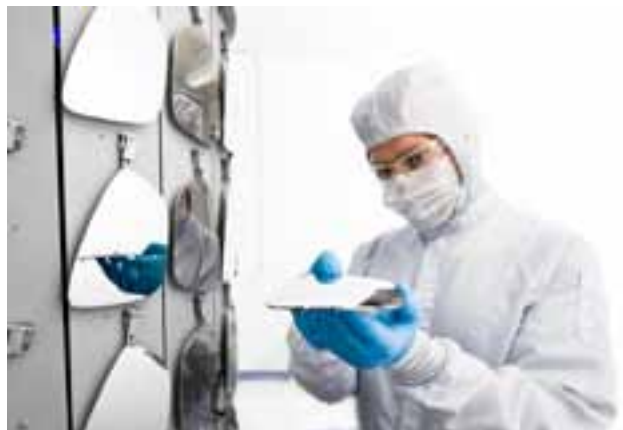
Nano technology is used to layer thin coatings over the polycarbonate base to create the reflective surface of the plastic mirror face.
