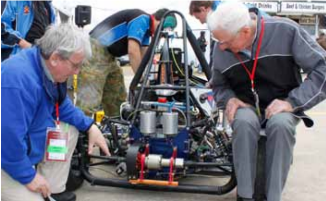
Design Patron Ron Tauranac AO (right) and I checked out the economical "bent pipe solid axle" technology used at both the rear and front of the University of NSW Australian Defence Force Academy car.
