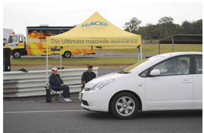
A comprehensive field test was completed to learn whether hybrid vehicles presented more risk than conventional vehicles to blind pedestrians.
