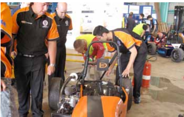
Figure 9> Deakin University team discovered that a spool drive does not work well with their “Sidewinder” chassis due to the centralised mass making it difficult to design in the required weight transfer.
