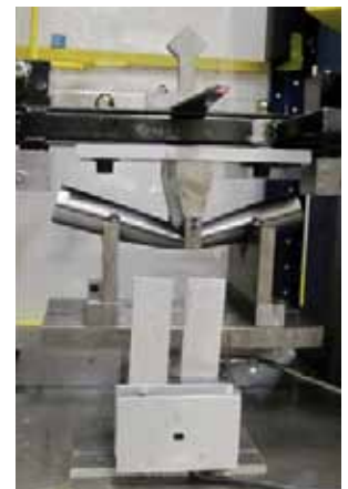
Figure 1 > The three-point bending rig using the drop weight test system.
