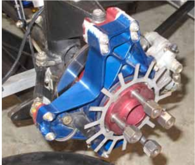
Figure 6 > This picture shows the workmanship in a rear suspension upright on the ADFA car. The de Dion axle can be seen, along with the toe control link and the Hall Effect wheel speed sensor, part of the traction control. It also shows some scuffing at the top of the upright caused by compliance in the assembly permitting contact with the wheel.
