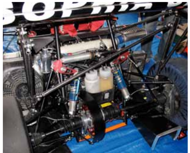
Figure 10 > Interesting features on the Sophia University car are the full length ground effects tunnels and the ride damper mounted between the suspension bell-cranks.
