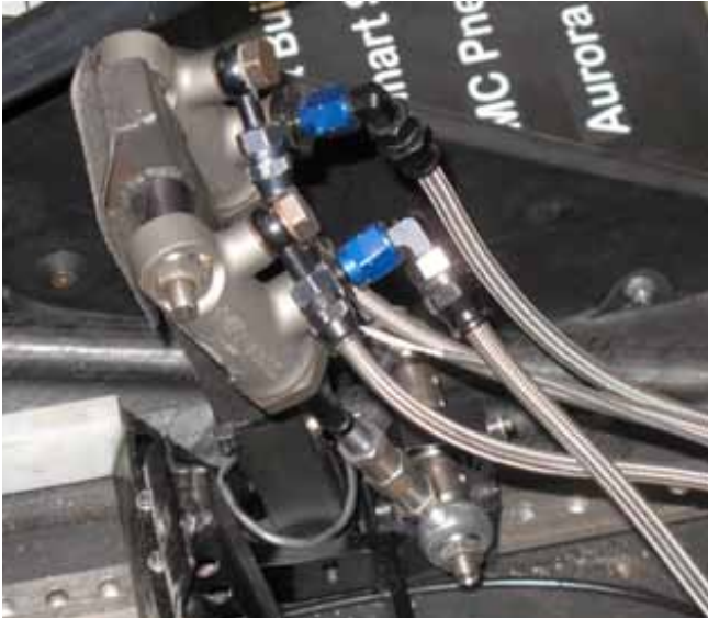
Figure 8 > The brake master cylinders on the Monash University car are mounted on a trunnion at the top of the pedal and on an adjustable balance bar at the bottom.
