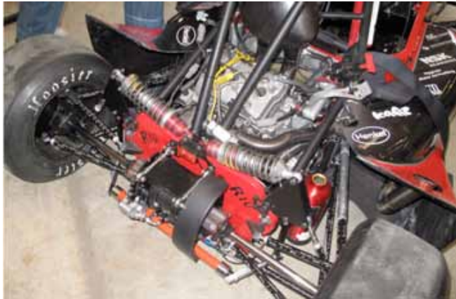
Figure 4 > The RMIT University internal combustion car featured a twin cylinder snowmobile engine.
