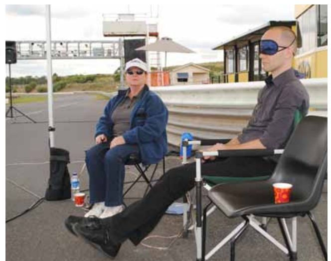
The audible approach of vehicles was measured by sighted subjects wearing blind folds and totally blind subjects. Part of the sound system playing back the replicated urban street sounds is seen at left.
