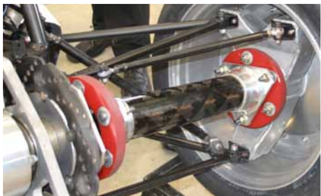
Figure 7 > Notable features on the University of Sydney car are the carbon drive shafts bonded to alloy flanges. The inner and outer couplings are polymer rings that will accept angularity, but which also absorb driveline snatch. The spun aluminium wheels, aluminium welded upright member and the scalloped inboard disk brake are all examples of the students' own work. Even the load paths in this assembly look good, something not always seen in a student designed car.
