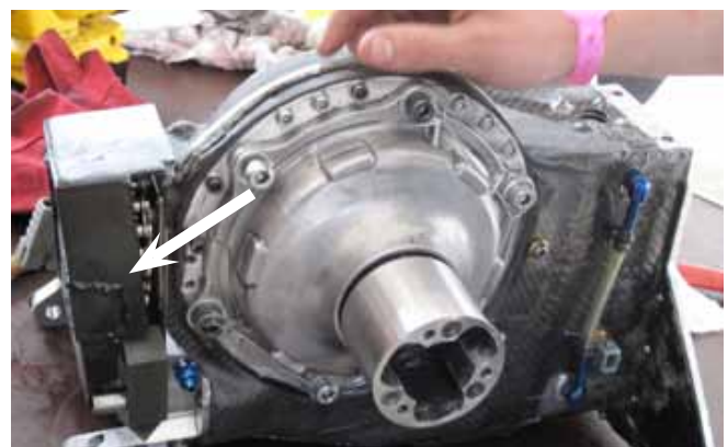
Figure 3 > A crack in the alloy transaxle housing (on the left), the chain drive and the tripod housings are shown here.
