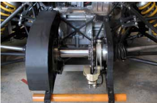
Figure 1 > The winning Monash University car shows off its spool drive. The simple structure can be seen with the drive sprocket mounted on one end and the rear brake disk mounted on the other. Cars fitted with differentials are usually fitted with two rear brakes to avoid braking across the differential.
