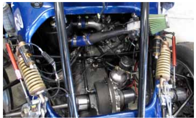
Figure 2 > The Auckland University drive train with student built carbon fibre transaxle. The Calspan decal represents the California test centre where a consortium of teams commissioned testing on tyres appropriate for Formula SAE.
